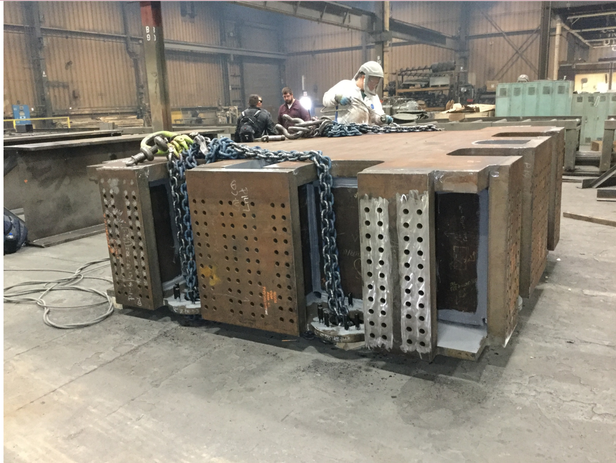
Type 7 Pedestal Fabrication in Wisconsin Shop
